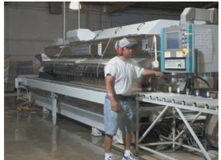
Aryeh’s first purchase when he opted to retool his shop was a multiple-head Comandulli polisher that’s proven to be a workhorse.
