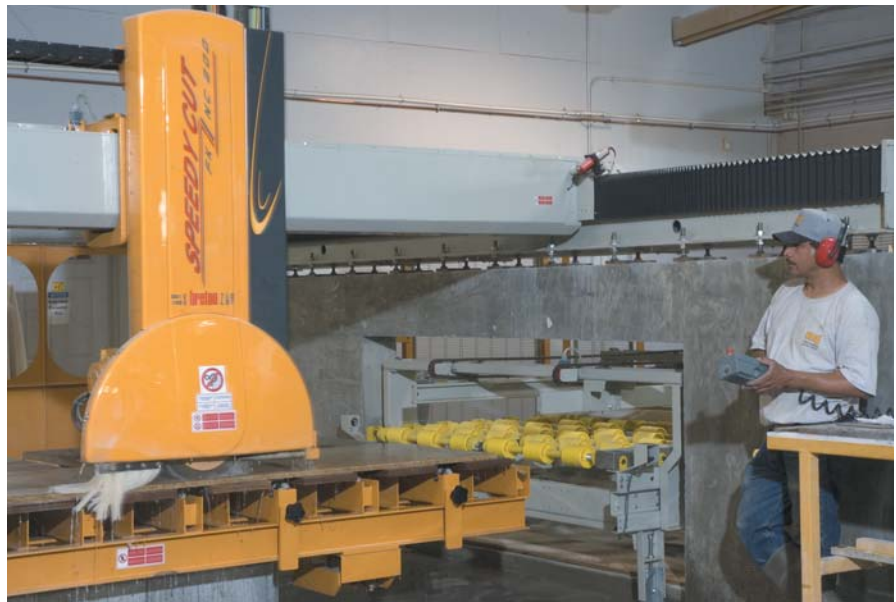
The company's five-table CNC bridge saw from Breton S.p.A accelerated the company's cutting times. Owner Aryeh believes technology allows his employees the time to put their craftsmanship to work where it's needed, rather than on more mundane tasks.
