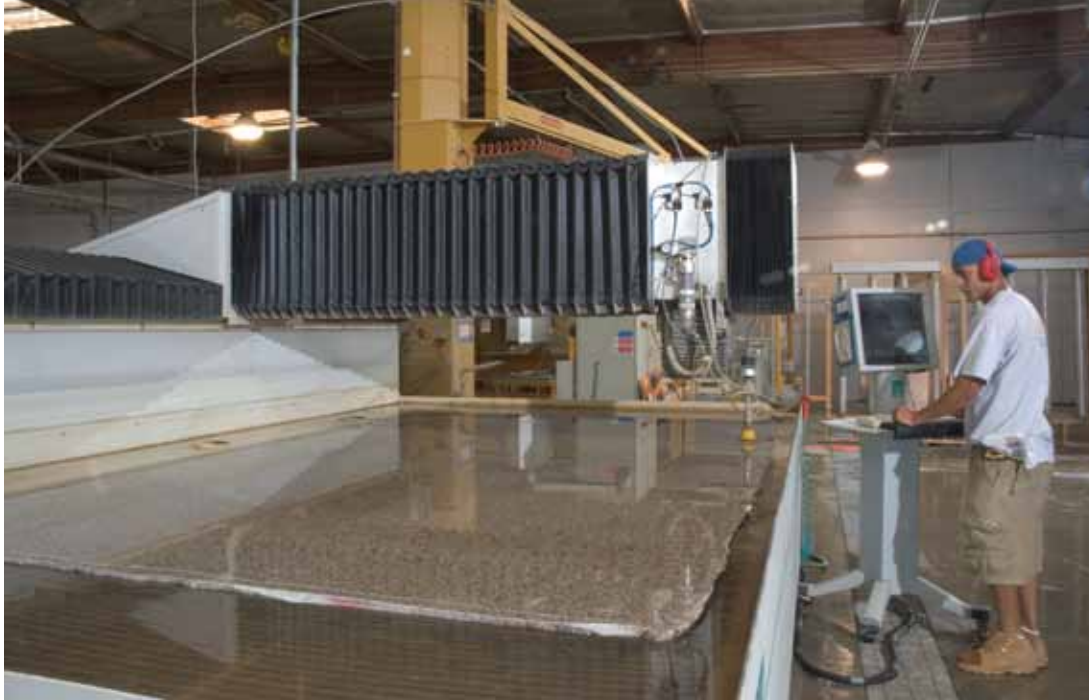
The waterjet allows SMG Stone to complete intricate stone pieces for high-end custom jobs.
