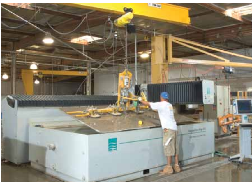
An Integrated Flying Bridge 6012 waterjet from Flow International of Kent, WA, was put in place because it can cut any material in any shape desired.
