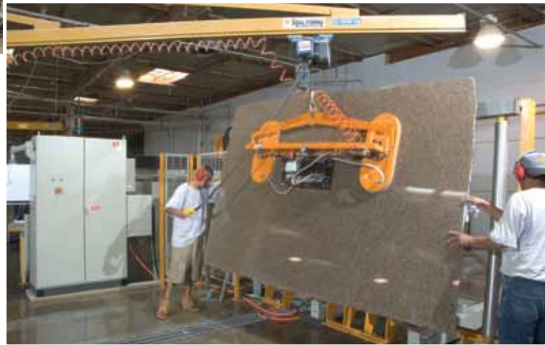
Workers utilize a Dal Forno crane and lifters to move slabs around the shop.
