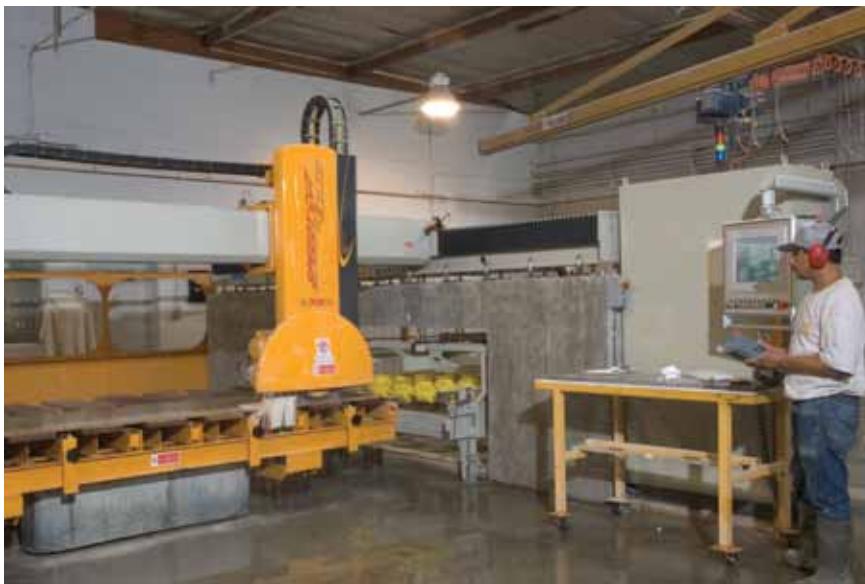
Among the machinery in the shop is a Speedycut FK NC/800 automated saw from Breton S.p.A. of Italy. “This is used for sawing slabs and blocks up to 10 inches thick,” said Solomon Aryeh, company owner. “It also is great for carving profiles, and it can turn columns with an attachment.”
